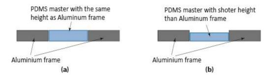
Fig. S1. (a) Using a PDMS master and aluminium frame with the same height results in thin COC chips (~100  $\mu$ m). (b) Thicker COC chips can be made by reducing the height of PDMS master.
