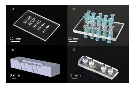
**Fig. S3.** a) CNC machined Plexiglas mold for casting PDMS ferrules. b) 0.8 mm needles are inserted in the holes so that the fluidic tubing feeds through the ferrule. c) Cross section of the Plexyglas mold, which is shown in (a). d) Actual PDMS ferule.
