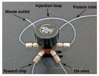
**Fig. S2**. A manual injection loop consisting of a LabSmith-MV303, 2 position – 6 port valve with 1/32 tubing was used for loss free sample loading.
