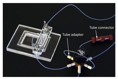
**Fig. S4.** COC chip and PDMS ferrule, mounted in CNC machined Plexiglas frame and connected to the 6-port, 2-position valve with injection loop. Only 2 of the 4 inlets into the chip are used in this chip design.
